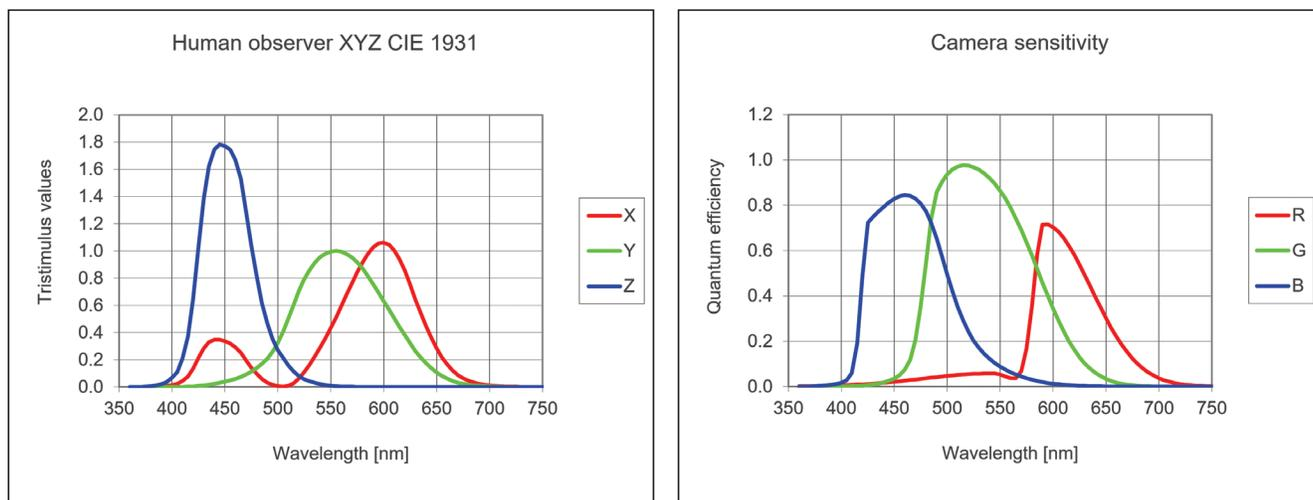
Figure 5. Left: color matching functions x, y and z (CIE 1931); right: camera sensitivity curves R, G and B (based on IMX214).
