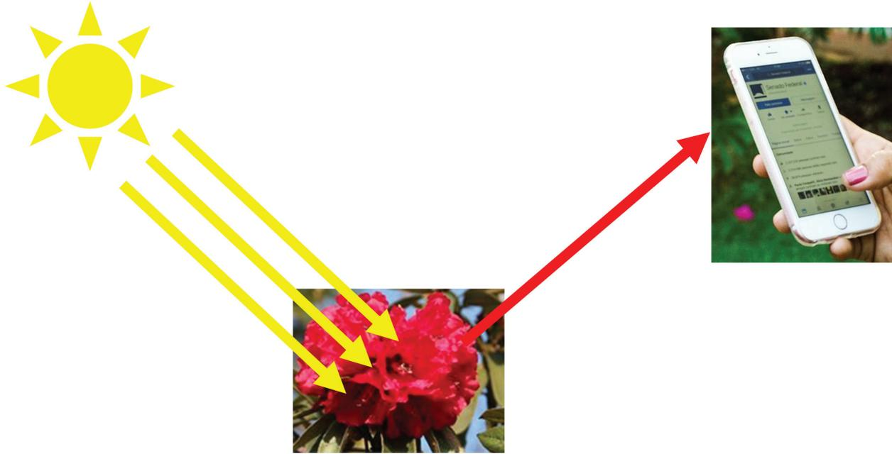
Figure 2. Elements contributing to the color reproduction – spectral properties of the light source, the reflectance properties of the object and the sensor spectral sensitivity.
