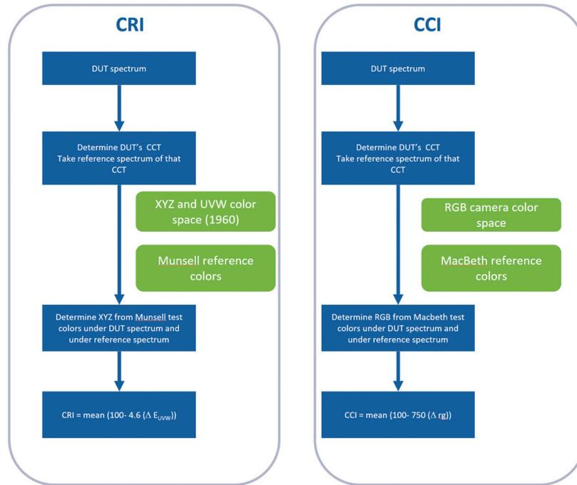
Figure 8. CRI vs. CCI procedure.
