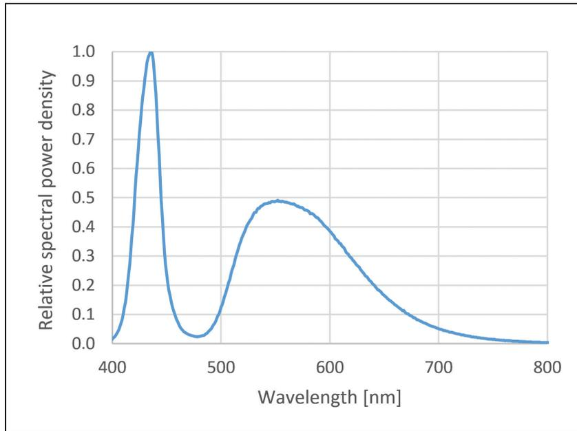
Figure 3. Typical white LED spectrum with blue pump and single YAG phosphor.
