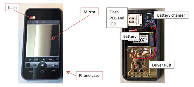
Figure 6. Camera flash for selfie demonstrator.
