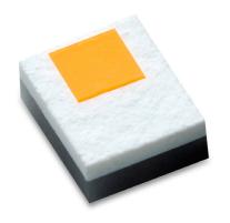
LUXEON FX LEDs with their Chip Scale Package (CSP) form factor are designed to meet present and future Automotive requirements. The Lumileds automotive binning structure meets both SAE and ECE color specifications and is hot binned at 85°C, consistent with actual automotive operational environments. LUXEON FX Plus PC Amber provides industryleading solutions for your front and rear turn applications. All LUXEON FX LEDs are IEC-60810 qualified.
