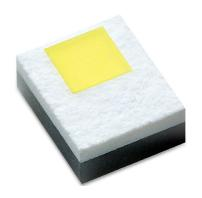
LUXEON FX Plus Cool White LEDs, with their Chip Scale Packaging (CSP) form factor, are designed to support low and high beam applications, daytime running lamps and front fog. The Lumileds automotive binning structure meets both SAE and ECE color specifications and is hot binned at 85°C, consistent with actual automotive operational environments. All LUXEON FX LEDs are IEC-60810 qualified.
