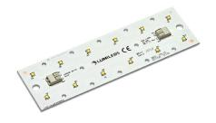
LUXEON XR-TX products are LED modules optimized for lighting applications requiring high efficacy LED arrays mounted on a rigid and thermally conductive substrate. These versatile building blocks feature 12 LUXEON TX LEDs on a MCPCB substrate, electrical connectors, and are designed for ease of system integration, faster time to market, and use with industry standard optics. LUXEON XR-TX will become a complete IP66 solution when used in combination with standard third party optics and heat sink.
