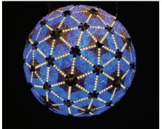
groups of four LUXEON K2 LEDs in red, green, blue, and white (RGBW). Each small triangle is fully isolated from its neighbors by reflective separation panels that prevent bleeding of light between triangles, allowing complete control of light color and patterns in the Ball.
